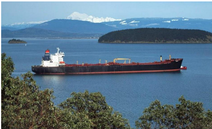
Kodiak (Exxon Ship). LOA 870 ft, beam 138 ft, draft: 45 ft. Displacement 150,000 tons in Puget Sound (Seattle, WA) April, 2010. New owner 2014.
