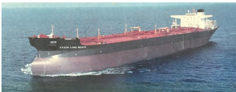
Exxon Long Beach. LOA: 987 ft, Beam 166 ft, Draft 64 ft. Speed: 16.0 kts. Displacement: 240,000 tons. New owner 2010
