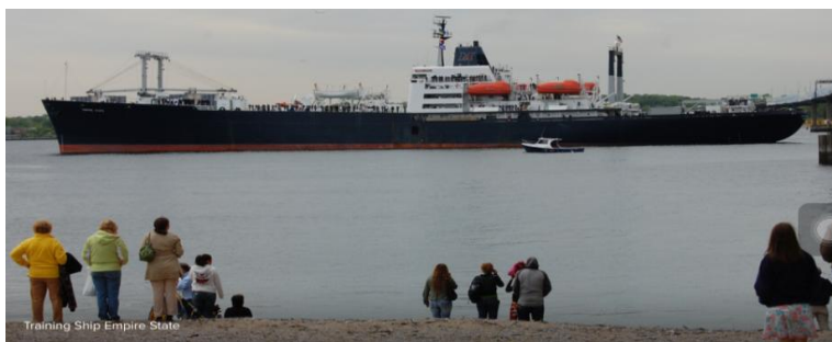
NY Maritime Training Ship Empire State VI. Displacement 17,000 tons. LOA 565 ft, Beam 76ft, Draft 25 ft., Speed 22 Kts
