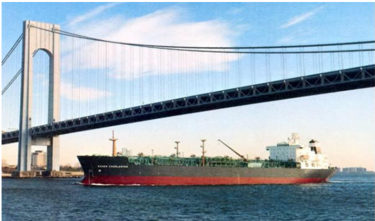
Exxon Charleston. LOA: 636 ft, Beam 106 ft, Draft 42 ft. Speed: 16.8 kts. Displacement: 62,500 tons. New owner 2004
